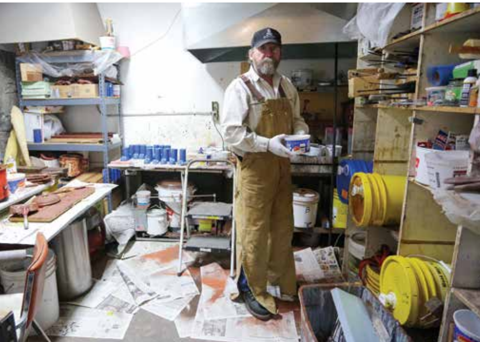
Smith prepares to measure out polyurethane for Tyrannosaurus rex teeth. The blue cylinders on the counter behind him are molds for those teeth.
